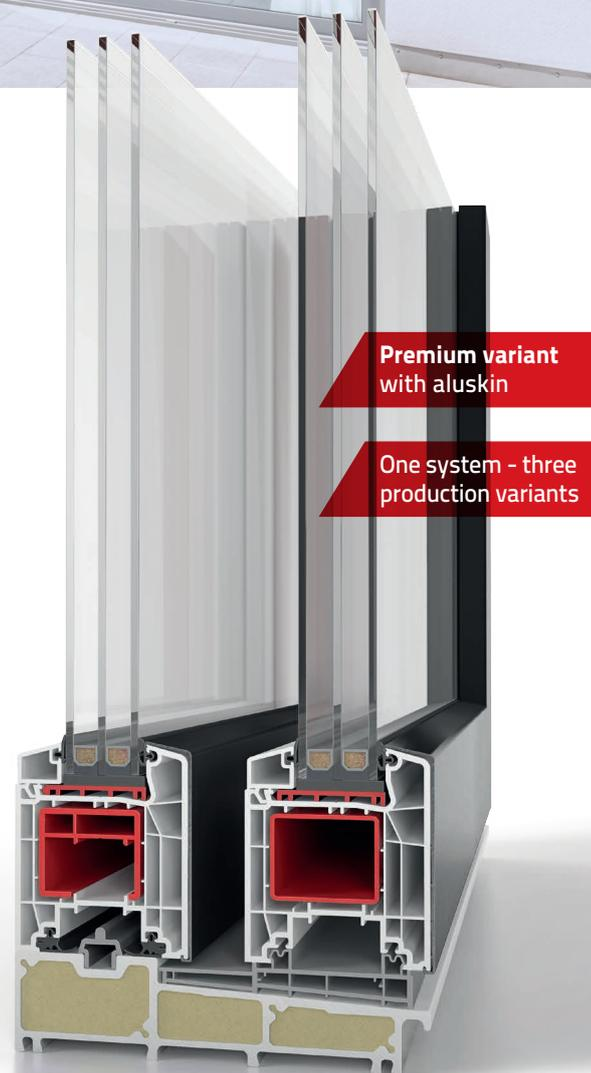
The Lift-and-Slide door delivers exceptional energy performance as standard. Ultra-energy efficient specifications, combined with glazing units of up to 51mm, deliver even higher levels of performance and U-values as low as  $0.65 \text{ W/m}^2\text{K}$ .
